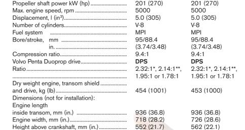
\* High altitude 1500 m (5000 ft) \*\* For special applications Propshaft power according to ISO 8665 Duty rating: R5 (Pleasure Duty)
